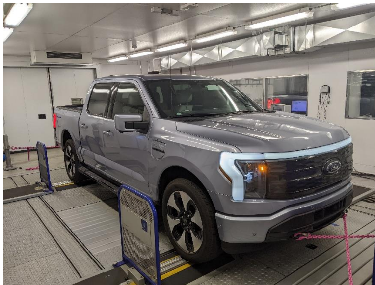
Figure 8: Ford F-150 Lightning on chassis dynamometer at the Automotive Research Center. Image Source: AAA
